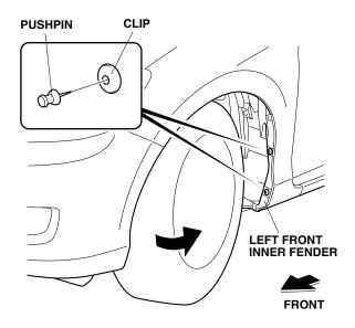
2. Using a pushpin, pierce the center of the two clips in the left front inner fender.
